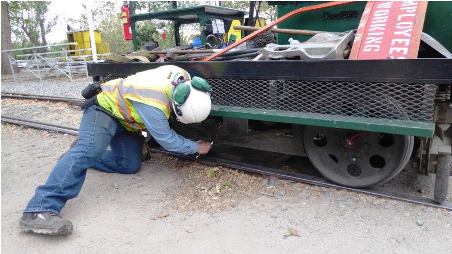
Joe working on the motorcar's brake-rigging
